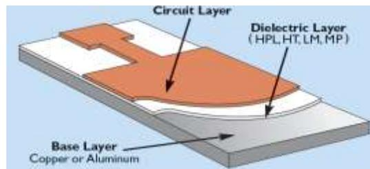
Optimal thermal management allows more forward current applied to the LED, which means increased light and potentially a reduction of LEDs required for the desired light specification. Supporting a cooler assembly with equivalent power equates to more light per die, and ultimately less dollars per lumen.
